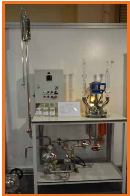
P.V.A. Pilot Tesisi Formaldehyde Pilot Plant
