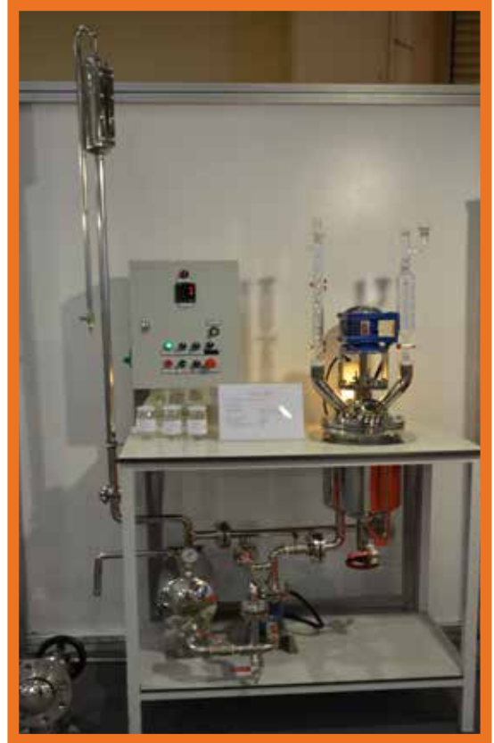
P.V.A. Pilot Tesisi Formaldehyde Pilot Plant
